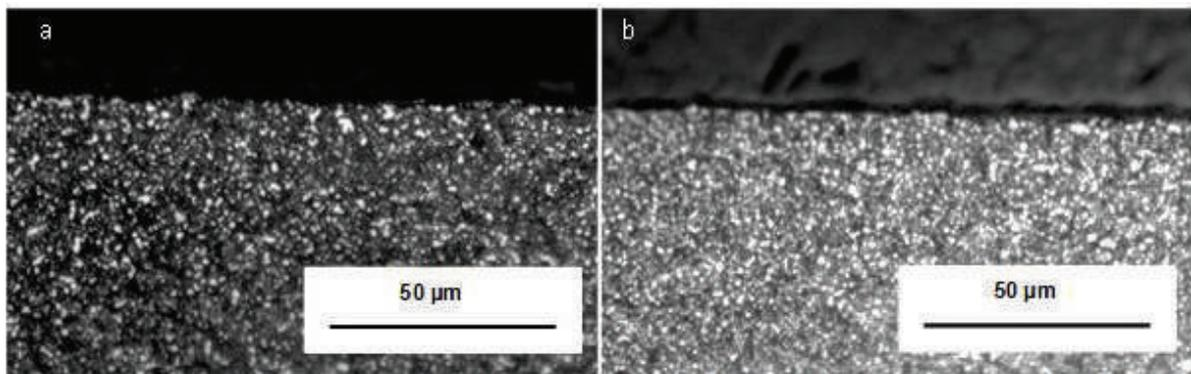
Fig. 6. Microstructure after turning with VCGW160408. (a) Dry machining; (b) CO<sub>2</sub> machining.
