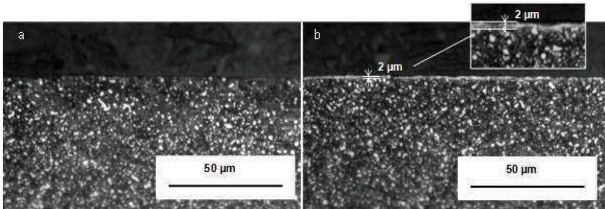
Fig. 5. Microstructure after turning with VNGA160408. (a) Dry machining; (b) CO<sub>2</sub> machining.
